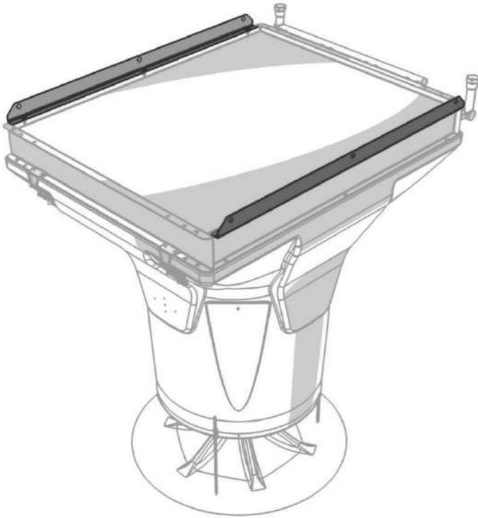
Distributor plate assembly for vertical flow installation
