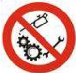
Prohibition of cleaning, oiling, greasing, repairing or adjusting moving parts by hand
