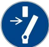
Obligation to cut power before starting work or repairs
